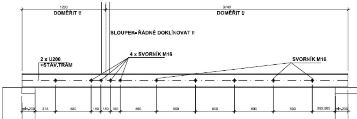
Figure 9 – beam steel liners
