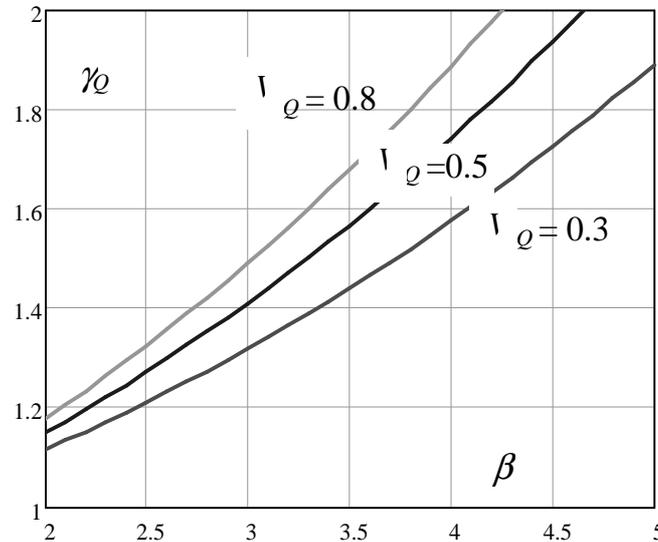
Fig. B.7. Variation of  $\gamma_Q$  with the reliability index  $\beta$  for selected values of the coefficients of variation  $V_Q$  assuming a Gumbel distribution of  $Q$ , period ratio  $N = 10$  and  $\alpha_T = 1$
