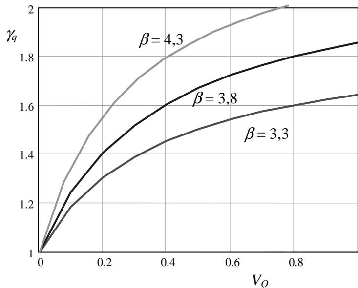
Fig. B.6. Variation of  $\gamma_Q$  with the coefficients of variation  $w_Q$  for selected values of  $\beta$  assuming a Gumbel distribution of  $Q$ , period ratio  $N = 10$  and  $\alpha_T = 1$
