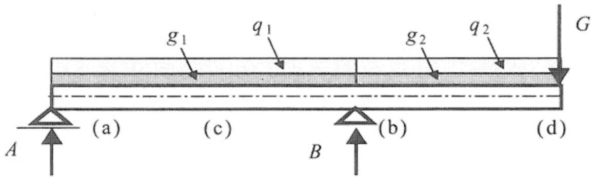
Figure 2: Beam with overhangs - assuming three independent permanent loads  $g_1, g_2, G$  and two independent variable loads  $q_1, q_2$ .
