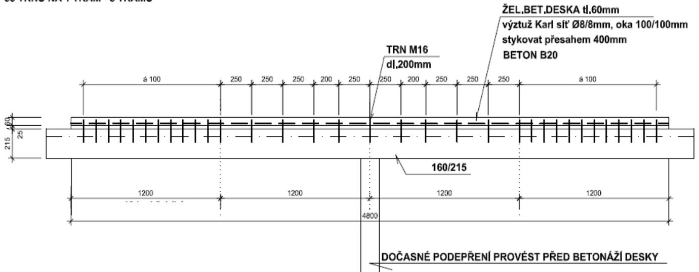
Figure 7 – beam- slab interconnection
