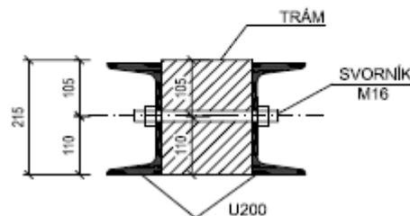
Figure 10 – beam steel liners - section
